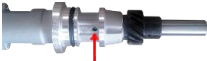
Drilled hole allows oil from the engine to lubricate the bushing
